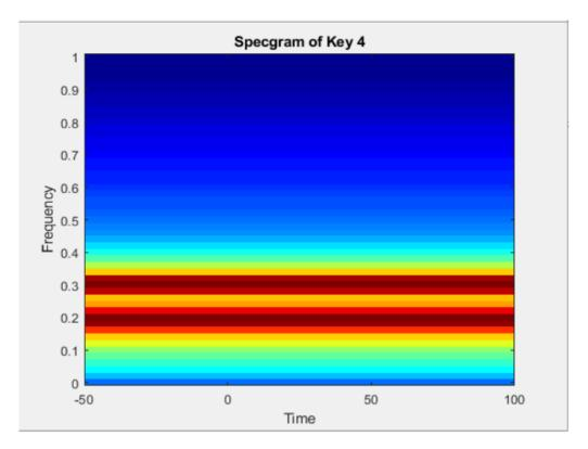
Here you have noticed that the low-frequency is very close to **0.2** along the normalized frequency axis (Brown color horizontal line) and the high-frequency is very close to **0.3** along the normalized frequency axis (another Brown color horizontal line). These numbers are estimated values.
