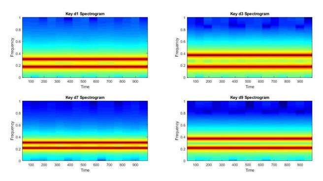
The spectrograms show the bands of frequencies generated for each digit used. We have two frequencies for each digit used.
