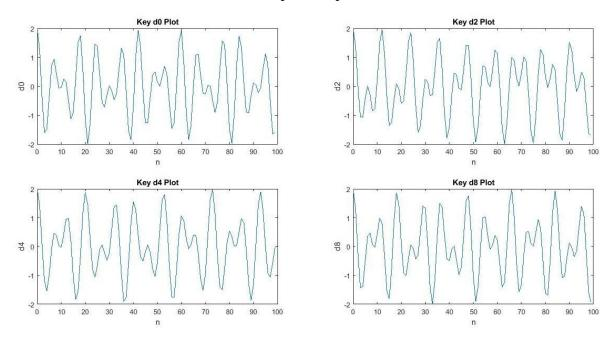
The graphs show the samples that are taken for each digit based off of the Cosine equation in the step 2. The amplitude of the plots is between -2 and 2. The samples are between 0 and 100.
